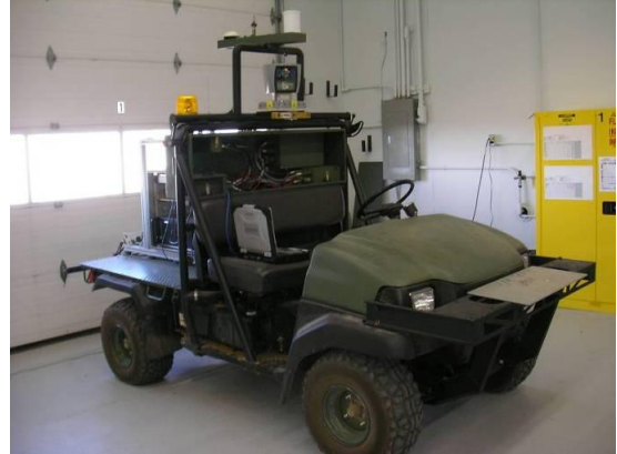
Fig. 3. Research platform used to conduct the tests. The Velodyne lidar and the Point Grey Research stereo camera housed on top of the vehicle were used for all tests.
