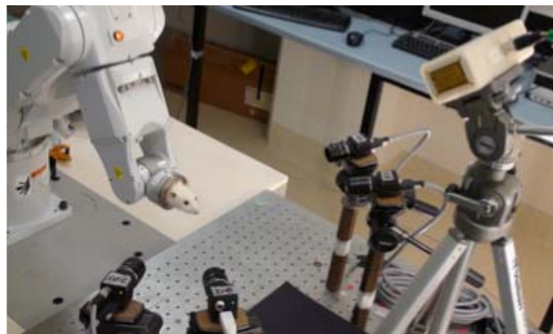
Fig. 2. Photo of the setup for validation showing the four cameras arranged in two pairs, and to the right the MicronTracker which was used for marker-based tracking.
