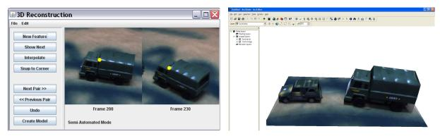
Figure 4 Semi-automated 3D reconstruction GUI (left) and the resulting 3D model visualized in ArcGlobe (right).
