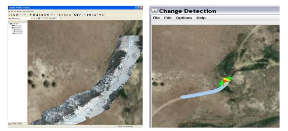
Figure 3 A high resolution mosaic overlaid on a lower resolution reference map (left). Change Detection GUI where the colour flags indicate the different types of changes (right).
