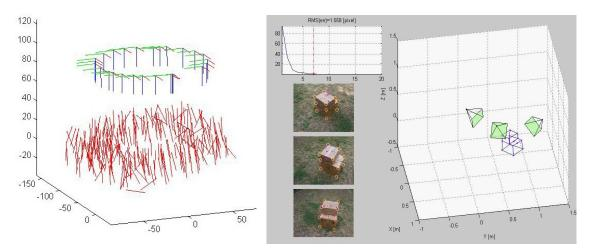
Figure 1 MV-SLAM output including the key pose trajectory and the features (left). Multi-frame bundle adjustment showing the match points in the left three thumbnails and the reconstructed structure on the right (right).
