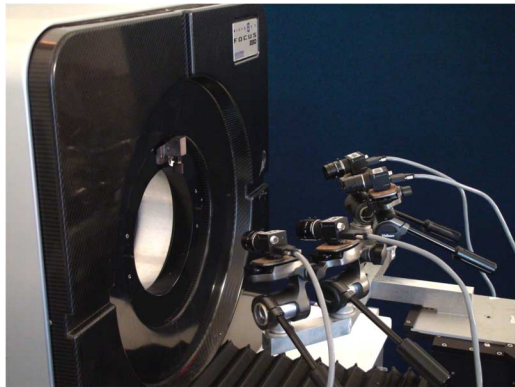
Fig. 6. Integration of the markerless tracking system with the Focus 220 scanner.
